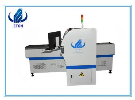
Apply to the 0.6M,0.9M,1.2M hard light board and 0.5M, 1M LED soft lamp strip. Producing with 2-4 types of materials with high capacity, available for board with any proportion of LED chip and resistor. Two mounting part, 17 nozzles for each mounting part, part A or part B can be mounted separately or synchronously.
