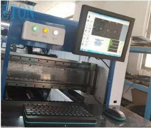
Our pick and place machine HT-E5D is very good per performance, it is dual system, dual module multifunctional mounter machine, there are two conveyor, so it can produce two different products at same time with high capacity. And HT-E5D is high precision, which reach 0.02mm, cause the X axis is magnetic liner motor, Y axis and Z axis is servo motor.
