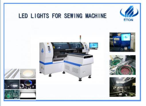
HT-T7 led lamp machine ,XY Axis running mode adopts the imported Linear Guide Rail and Ball Screw to ensure the mounting accuracy within 0.01mm.Linear Guide Rails coordinating with Ball Screw to ensure long-term quick positioning, low noise and high precision.
