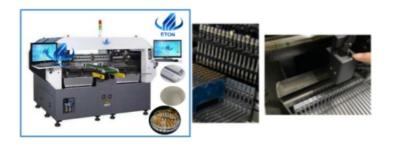
COMPONENT: Min.size 0603 L\*W\*H:2700\*2120\*1550 mm PCB L\*W:250mm \* any length
