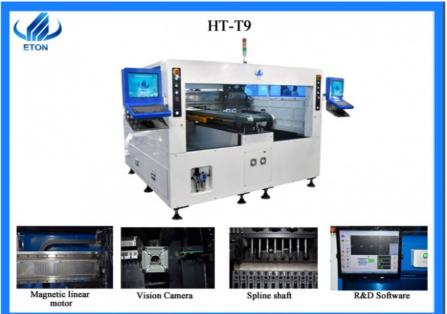
Producing with 2 4 types of materials with high capacity at same time. Single plate material can be mounted, and the same plate material is always mounted on the same lamp. Dual-arm four modules with 16 nozzles for each mounting part, and part A/B/C/D can be mounted separately or synchronously. Calibration automatically. Exclusive patent technology:group to pick and group to mount.
