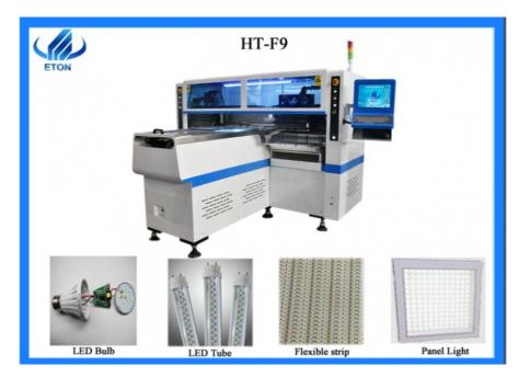
HT-X9 is dual-arm magnetic levitation LED high speed pick and place machine.the capacity reach 200000CPH.It is Suitable for 0.5M,1M Strip, Tube and Panel Light.it can mount LED 3014/3020/3528/5050 and resistor,capacitors,bridge rectifiers,etc.
