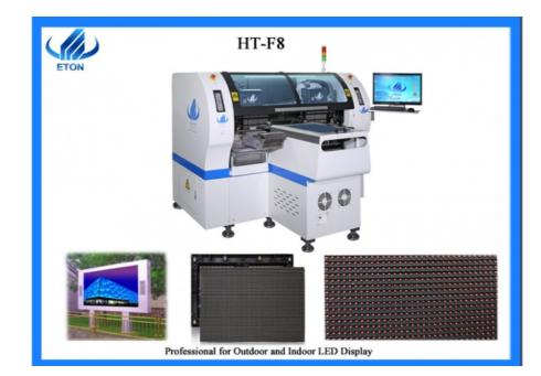
Components of pick and place machine ht-f8 can mount include LED2121/2727/3528/5050 and resistor, capacitors, bridge rectifiers, etc.
