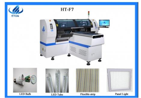
Components of this high speed SMT mounter machine ht-f7 can mount include LED3014/3020/3528/5050 and resistor, capacitors, bridge rectifiers, etc.
