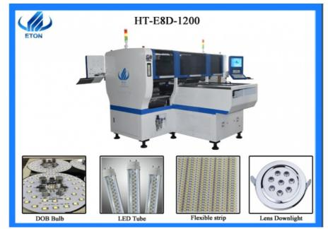
HT-E8D machine is Dual system, dual module multifunctional mounter with high capacity of 80000CPH. It can mount capacitors, resistors, LED3014/3020/3528/5050, IC and shaped components. It applies to power driver, electric board, lens, linear bulb, household appliance and etc.
