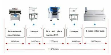
Step one: Using Solder printing machine to Print Solder paste on PCB.
