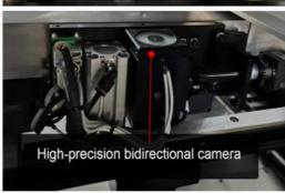
High-precision bidrectional camera, including reflective prism, can be illuminated up to the steel mesh, down to the PCB board.
