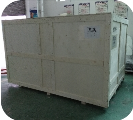
Step 4. customized Strong wood carton packing The customized strong wood packing for ocean ship, The machines are fix oin the wood carton, effectively prevent collision and shock.
