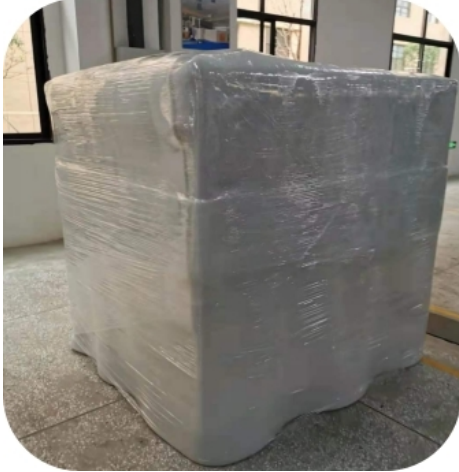
Step 3. Unique tin foil packaging Add tin foil packaging can prevent the film from scratch broken.
