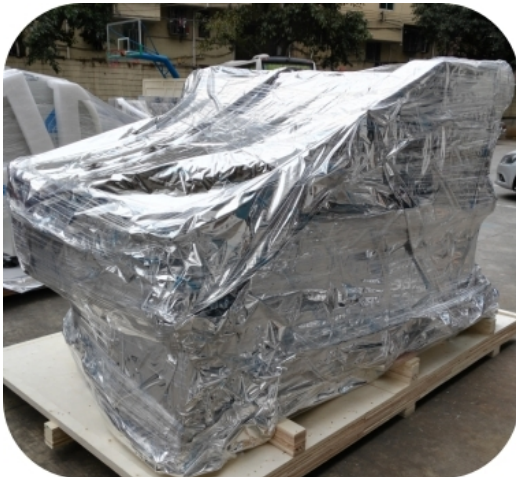
Step 4. customized Strong wood carton packing The customized strong wood packing for ocean ship, The machines are fix oin the wood carton, effectively prevent collision and shock.
