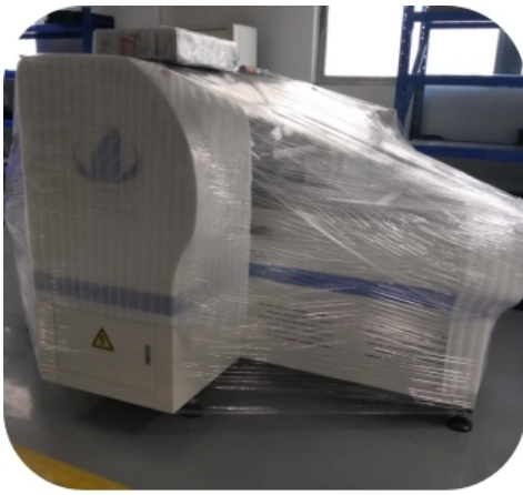
Step 2. Add foam+film packaging Double safe protection, Prevent the machine from crash and shaking
