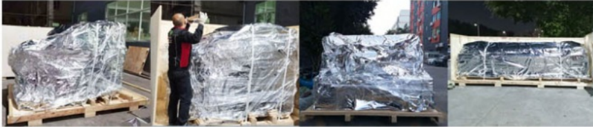
Step two: Vacuum packaging Vacuum packaging; put the desiccant in a vacuum bag to prevent moisture; use straps to secure the machine;
