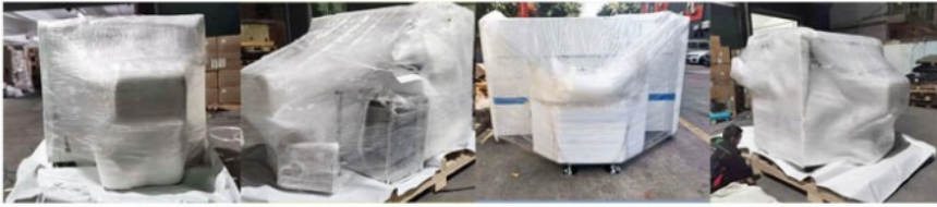
Step one: Pack the machine with foam cotton and stretch film to protect the outside of the machine
