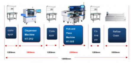
Glue dispensing machine, conveyor, Pick and Place machine, reflow oven.
