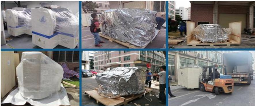
**Step 1: Film packing and foam cotton prevent the dust and water to protect the machine;**
