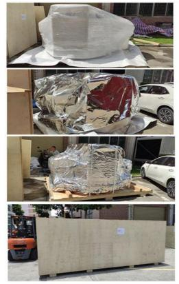
Step1: Wrap with stretch film to prevent the equipment from
