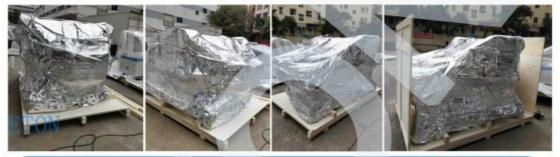
Step two: Vacuum packaging:put the desiccant in a vacuum bag to prevent noisture; use straps to secure the machine
