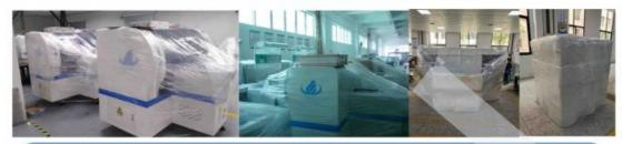
Step one: packing the machine with foam cotton and stretch film to protect the outside of the machine
