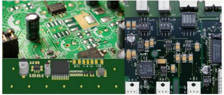
1.PCBA process: PCBA = Printed Circuit Board Assembly, that is, empty PCB through SMT, then DIP plug-in through the entire process, referred to as PCBA process.
