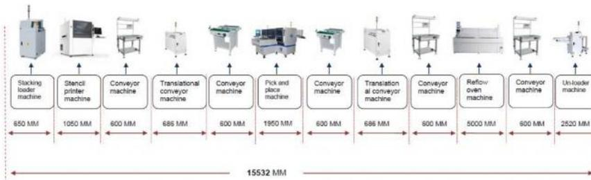
SMT production line main equipment: Printing Machine, SMT machine, reflow soldering, wave oven, Prospect
