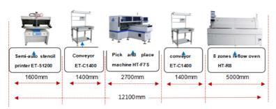
HT-F7S high-speed semi-automatic line of LED lamp tube optimal production capacity: 150,000-170,000 CPH actual production capacity: [3600 sec/(in and out of the Board 8 sec + full-page Patch Cycle Times + 1 sec)] \* single board material quantity \* splicing quantity = about 130,000 CPH
