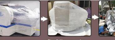
Step 1: Film packing and foam cotton prevent the dust and water to preotect the machine; Step 2: Vacuum package and moisture proof bag, to keep dry of the machine during transportation;
