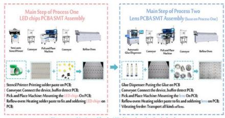
(One smt machine is used for the LED chip and another for the lens)
