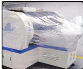
Step 1: Film packing and foam cotton prevent the dust and water to protect the machine;
