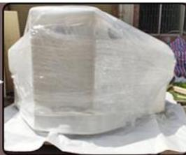
Step 2: Vacuum package and moisture proof bag, to keep dry of the machine during transportation;
