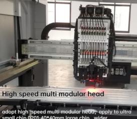
adopt high speed multi modular head, apply to ultra small chip 0201-40\*40mm large chip, wider component range
