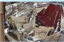
Step 2: Vacuum paper packaging and moisture-proof bag so that the machine can be kept dry during transportation to prevent moisture
