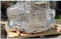
Step 3: Use straps and triangular wood to fix the machine to prevent damage to the machine during transportation
