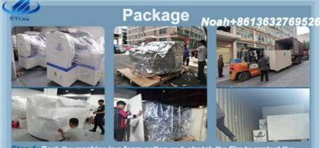
Step 1: Pack the machine in a foam cotton and stretch the film to protect the outside of it. Step 2: vacuum paper package and moisture proof bag, to keep dry of the machine during transportation to prevent moistrue. Step 3:Each exported machine will be equiped with sturdy wooden boxes, to ensure the safety of the machine. Step 4: Transportation by trucks to the specified port. For the feeders and some spare parts usually we'll pack it separately with box.
