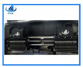
From this picture, we could see there are two mounting modules, and each mounting module are 17 heads. The mounting way is group to take and group to mount, very fast, can reach 170000 chip per hour.
