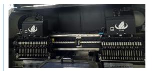
Feeding way: Electric feeder with double motor
