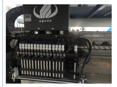
Two mounting modules 16 Nozzles and 32 Electric feeders for each mounting part
