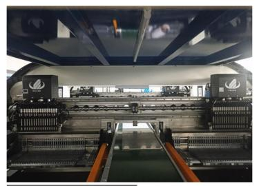
PCB carrying mechanism PCB length and width: 250mm\*any length PCB clamping: Adjustable pressure pneumatic Conveyor Transmission: Belt drive Transmission
