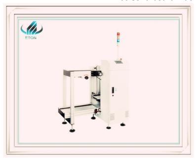
The SMT board machine is a kind of production equipment used in the SMT production and processing of electronic products. Its main function is to put the unmounted PCB board on the SMT board machine and send it to the suction machine, then the suction board. The machine automatically places the PCB on the track of the solder paste printer and uploads it to the solder paste printer for brush solder paste operation.
