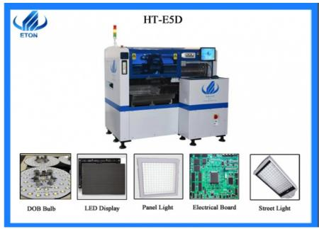
HT-E5s machine is single module multifunctional mounter with high capacity of 40000CPH. It can mount capacitors,resistors,LED3014/3020/3528/5050,IC and shaped components. It applies to power driver,electric board,lens,linear bulb,household appliance and etc.
