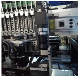
Mark camera: Do PCB board placement procedures.
