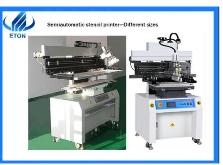
Semiautomatic stencil printer machine is very flexible, suitable for different pcb sizes products, such as the led tube, bulb, strip light, driver board, etc. It is easy to change the stencil for different board.
