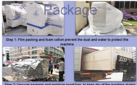
Step 2: Vacuum package and moisture proof bag, to keep dry of the machine during the transportation, then equip with sturdy wooden boxes and transported by trucks to specified port
