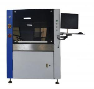
RT-2 pick and place machine: Accurately install the surface assembled components to the fixed position of PCB.
