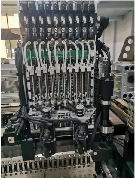
Screw rod:The function of the screw rod is to convert the rotary motion of the servo motor into linear motion, so as to drive the mounting head to move back and forth on the linear guide rail to mount components.
