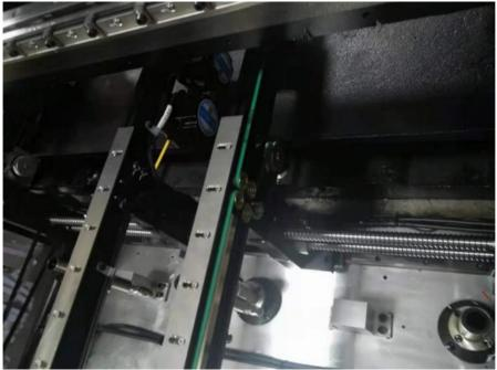
Drag chain:Wrapping the line to ensure the translation of the line. Reduce wear and prolong service life.
