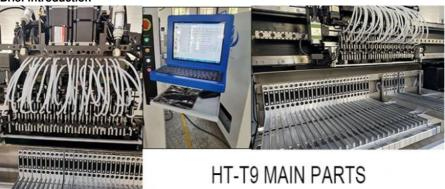
(1)Most of our customers are interested in why this machine can reach so high speed. You know it called mounting module. HT-T9 also has two modules, but one module has 2 mounting parts and each mounting parts has 17 heads. Totally 68 mounting heads. That make HT-T9 can pick and place components such quickly. This is the main reason why HT-T9 can reach 250000CPH and get higher mounting speed.
