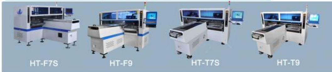
3. HONOR series pick and place machine, apply to 0201~40\*40mm tape reel package and IC tray feeder, adopt new feeding way, docking cart, IC tray feeder and double head intelligent feeder
