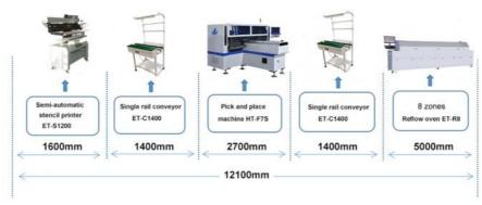
Stencil Printing: solder paste is a follow-up material for the surface adhesive components and PCB to connect with each other. First, the steel plate is etched or laser cut, and then the solder paste is printed on the welding pad of PCB by the squeegee of the Printing machine, so as to enter the next step.
