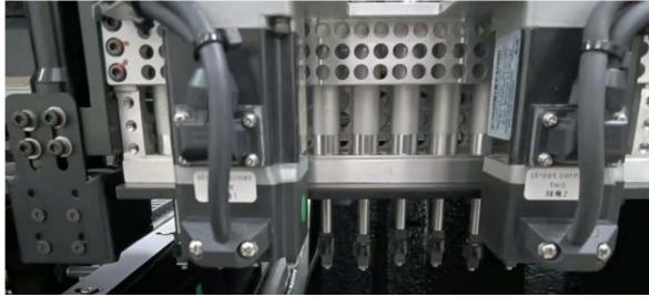
The electromagnetic valve: The mechanical movement of the suction nozzle is controlled by controlling the on-off current of the electromagnet.
