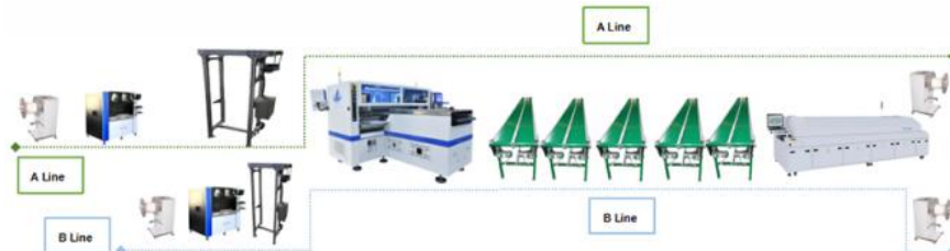
T9-2S two belt line smt production
