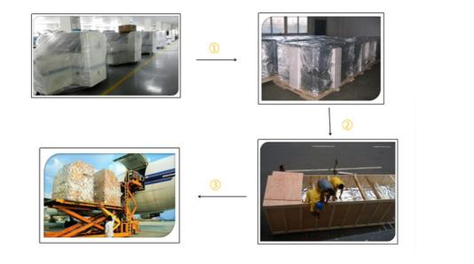
All machines are packed with vacuum and wooden packing like the one in the pictures. Step1:Film packaging. Step2:Vacuum packaging. Step3:Wooden box packaging
