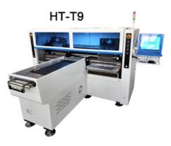
Dual arm magnetic linear high speed mounter for flexible strip(no wire), Producing 4 types materials at the same time capacity reach 250000 CHP.
