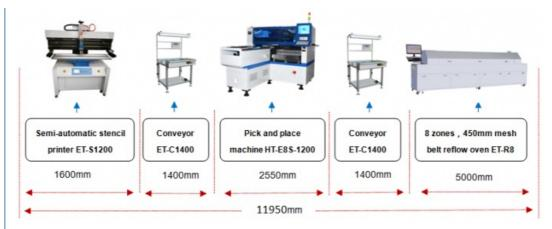
We have full range of pick and place machine production line equipment, So we have the professional suggestions for you to build the production line.
