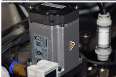
▲ X,Y,Z DRIVE WAY Magnetic linear motor Servo motor
