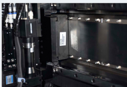
▲ X,Y,Z DRIVE WAY Magnetic linear motor Servo motor
