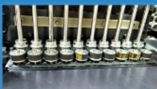
10 Heads rotation angle controlled by 10 PCS independent motor, more flexible mounting solution
