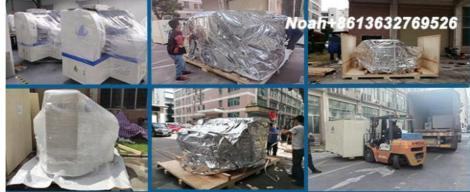
Steep 1: Film packing and foam cotton prevent the dust and water to preotect the machine;
