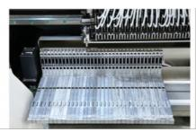
Adjust the conveying platform according to various roll to roll strip, range 250±10mm, the max length range is 1M per cycle.
