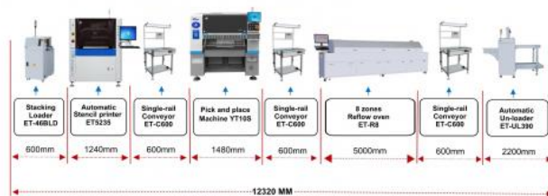
ETON –YT10S Full-Automatic Production Line
