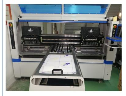
Dual-purpose professional high-speed attaching machine, 2 ~ 4 type capacity of 150000-180000CPH. Visual alignment, mark correction.
